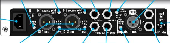
**IMPEDANCE SELECT** for tailoring the preamp input impedance to your specific pickup.
