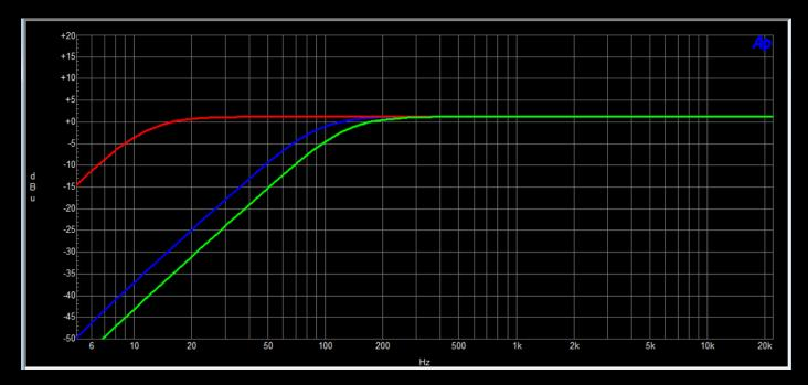
Red = Without HP filter. Blue = 80Hz HP filter. Green = 120Hz HP filter.
