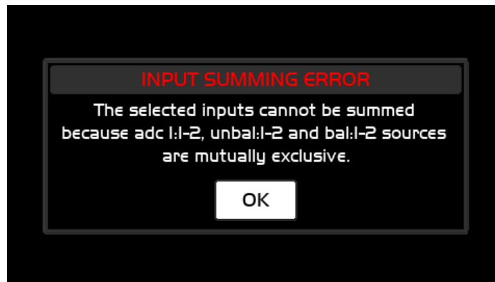
Illustration 16: Input Summing Error: ADC1 1-2 bal-unbal
